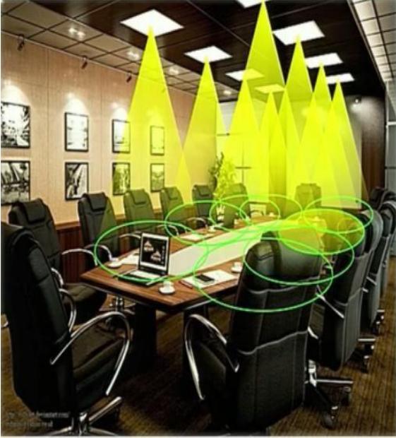
Fig. 1: - Use of LED illumination as a transmitter
