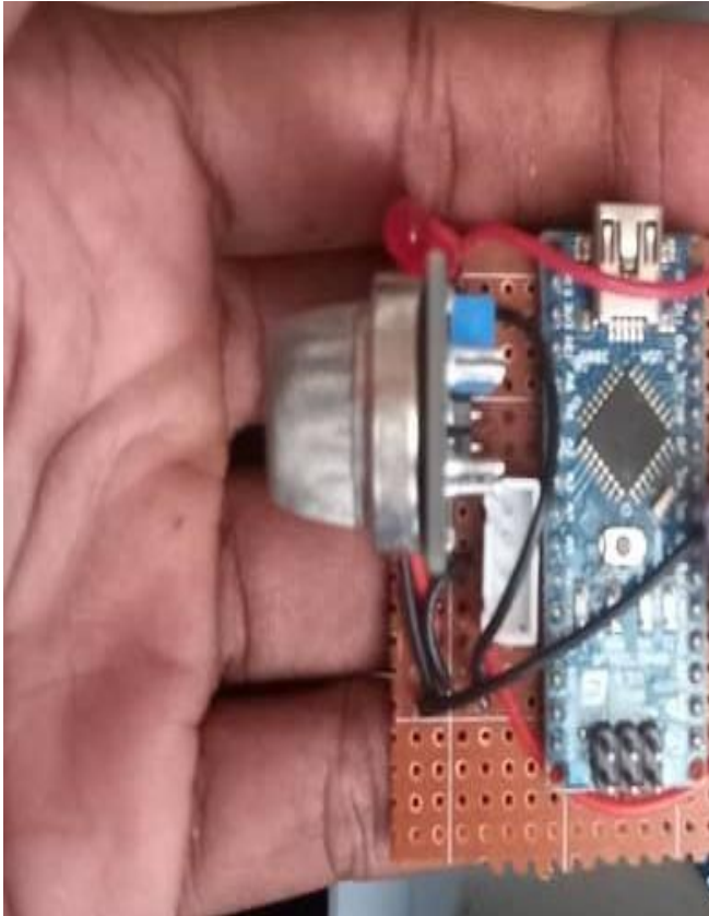
Fig. 4. Circuit built on the Vero board
