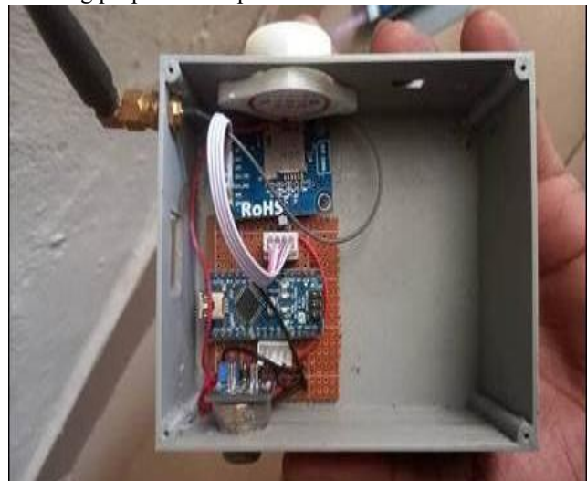
Fig. 7. Installation of components into the casing
